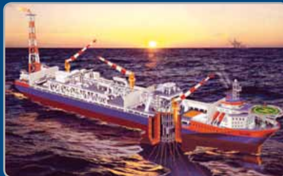
Floating production unit (FPSO)
